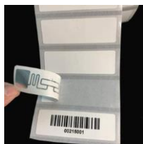
Example of a Smart Label that prints barcode and RFID
